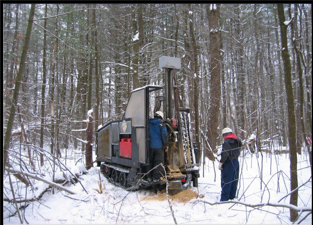
Figure 3 Low impact seismic drill.
