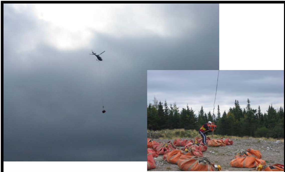
Figure 5 Helicopter being used to move geophones.
