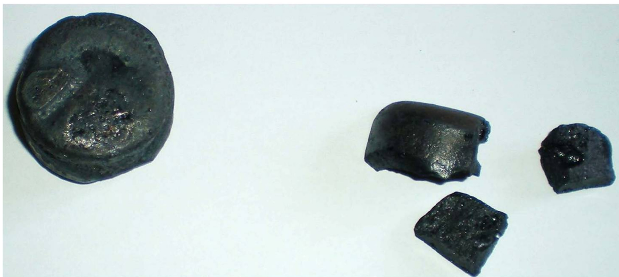
Photo 6 Pig iron piglet and slag produced from Churchill River iron ore in 2006
