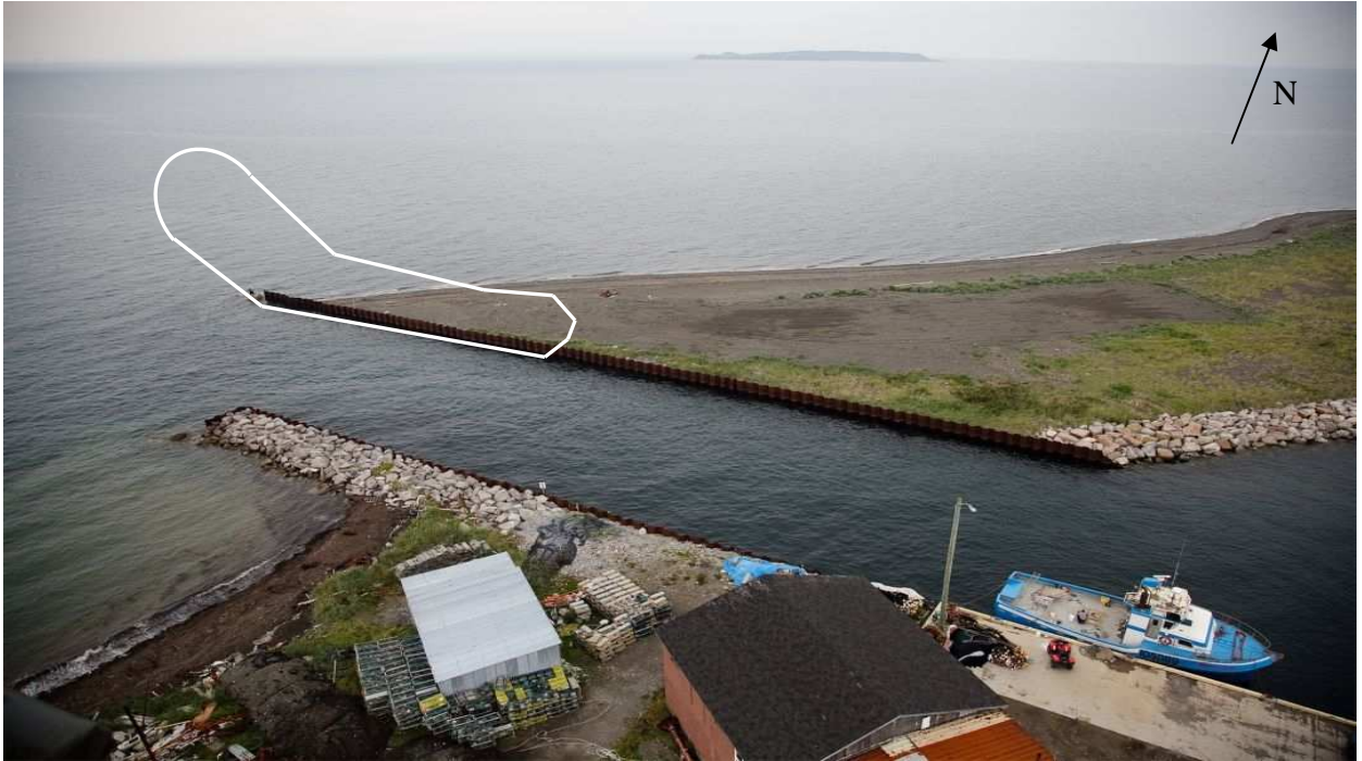
Appendix A-3. Phase 1: Channel wall reconstruction and breakwater construction. * Illustration not to scale.
