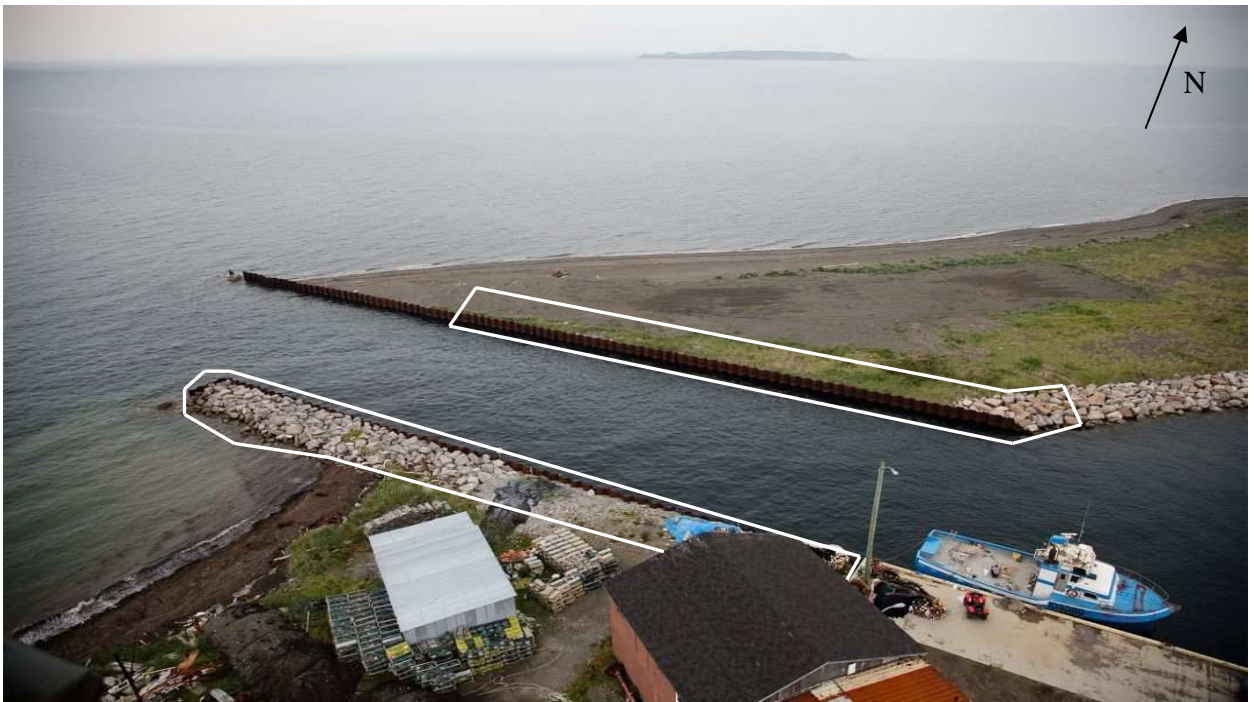
Appendix A-6. Future phases: Armourstone protection installation (north and south side). *Illustration not to scale.
