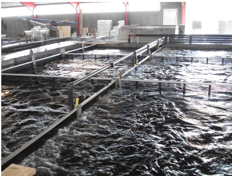
The moving bed bio filter, see table for specifications
