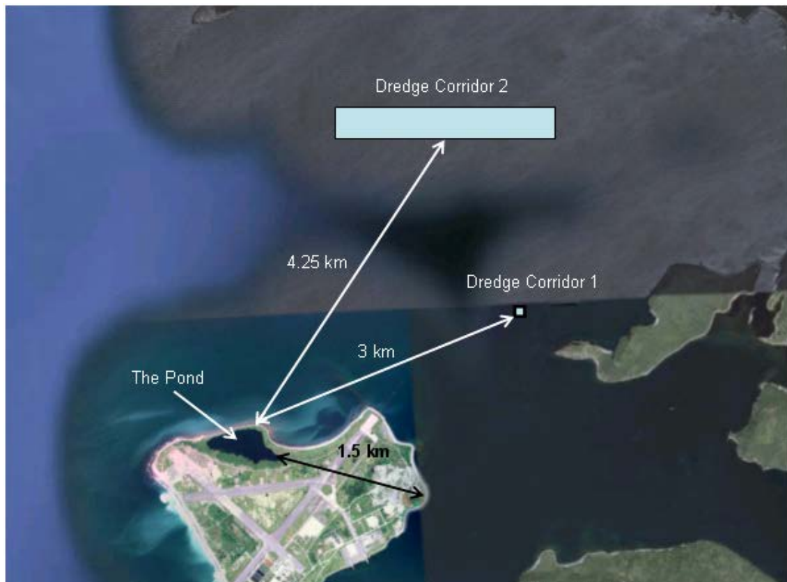
Figure 4-9 Corridors Requiring Dredging along the Concrete Gravity Structure Tow-out Route
