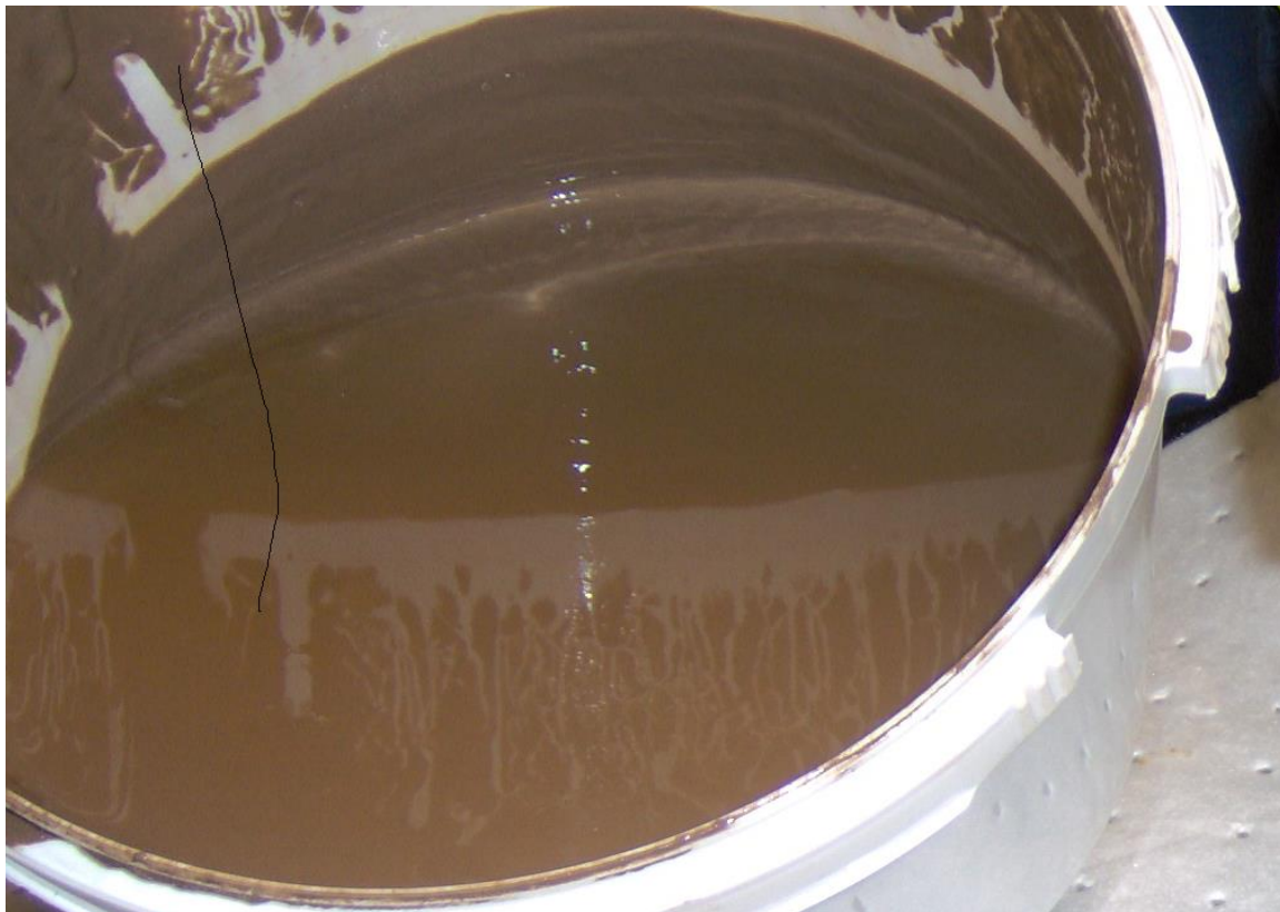
Picture 2. Centrifuged drilling mud/cuttings – also know as ‘underflow’
