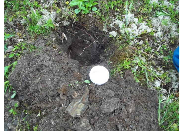
Test pit excavation for WABUSH3-SS2.
