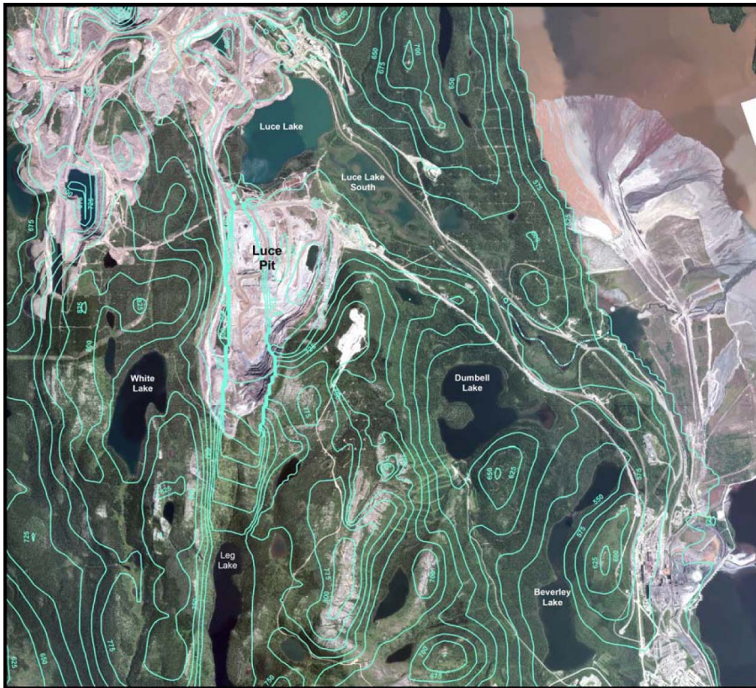
Figure 2. Model-predicted water table elevation contours for current (2013) baseline conditions prior to Wabush 3 mining (Luce pit dewatered to 540 m amsl).
