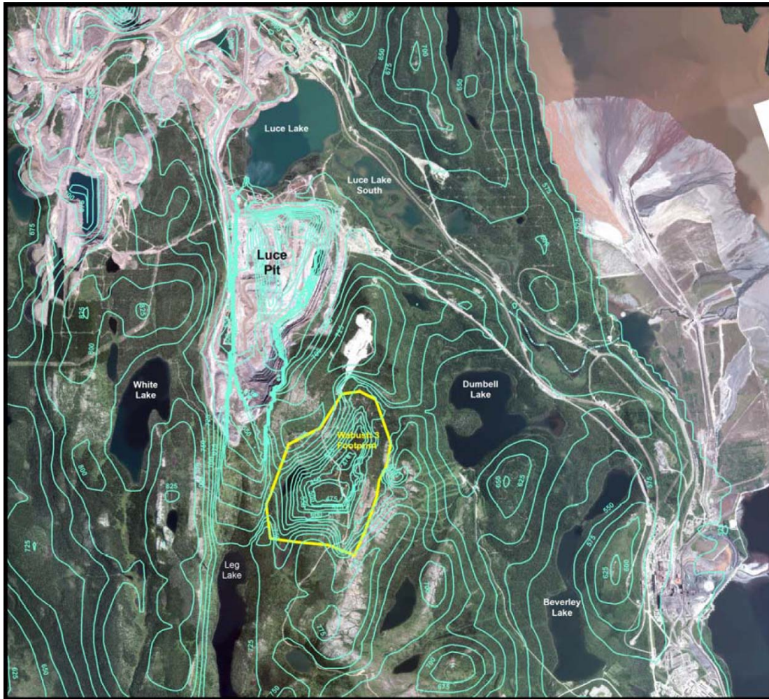
Figure 3. Model-predicted water table elevation contours at the end of Wabush 3 LOM in 2063 (simulation also includes Luce pit dewatering to 2063).
