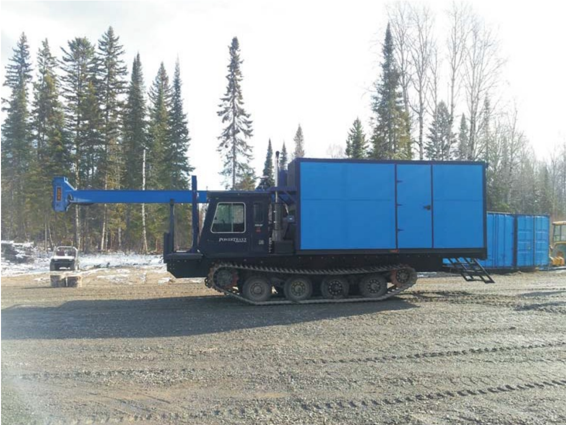
Figure 3 – Photos of two modern reverse circulation rotary drill rigs designed for till sampling
