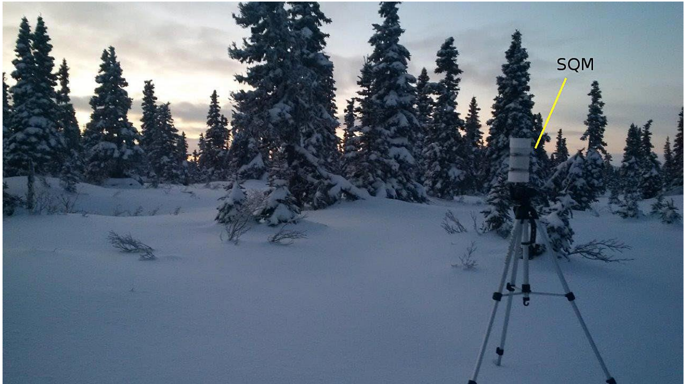
Figure 1 SQM-LU-DL with a protective housing mounted on a tripod. Credits: Denis Lalonde. AECOM
