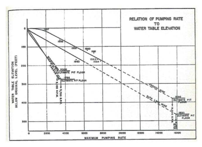
Figure 2-2 Relation of Pumping Rate to Water Table Elevation in Some Mines at Knob Lake Adapted from Stubbins and Munro (1965)
