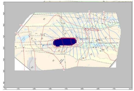
Figure 15: Groundwater drawdown during pit dewatering (SNC-Lavalin, 2015)
