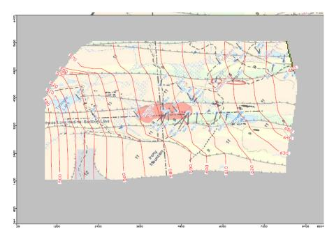
Piezometric Map during Pit Dewatering (Final Depth)
