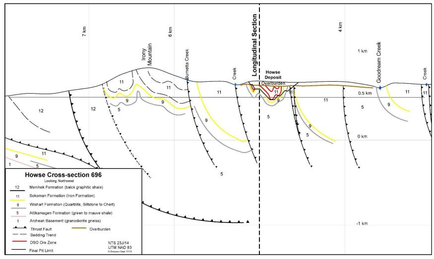
Figure 5: Howse Geological Cross-section 696 with the Profile of the planned pit
