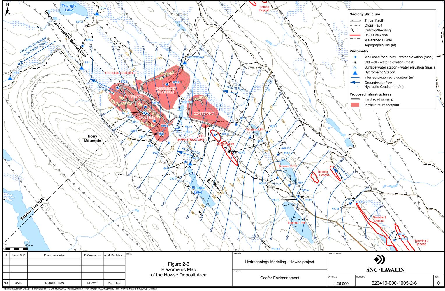
At the Howse deposit, the groundwater depth varied approximately from 39 m to 95 m below the ground surface. The local groundwater circulates in the fracture zones developed in some of the iron formations along the bedding plains and faults.
