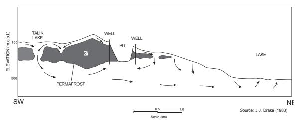
Figure 11: Groundwater Flow in a Region of Discontinuous Permafrost
