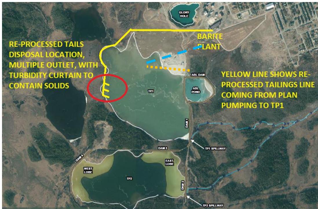
Figure 6 – Approximate locations of “oversize” (orange dashed Line), “Excess Water” (Blue Line) and Mill Tailings Line (Yellow Line)
