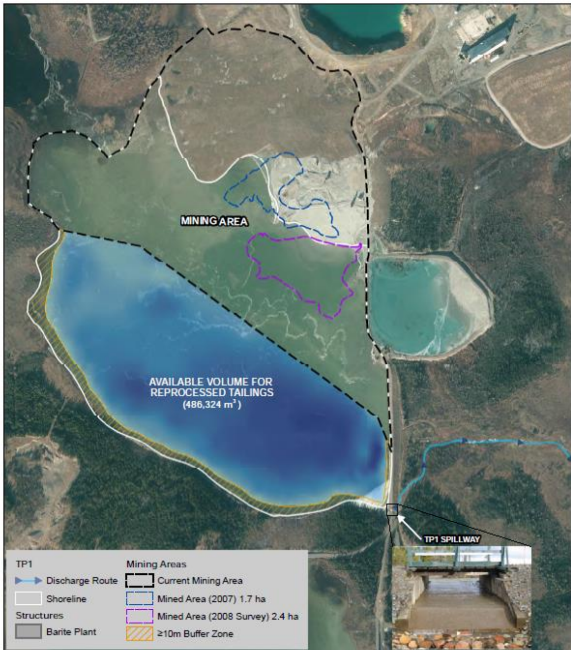
Figure 4 – TP1 showing spillway and proposed turbidity barrier location at discharge
