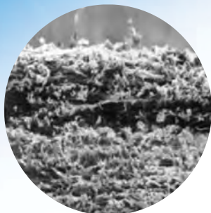
Commodity depth media loaded with ISO fine test dust
