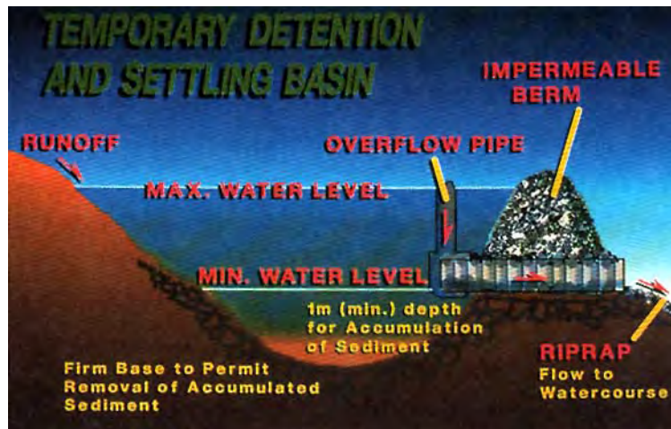
Figure 4.7 Features of a well-constructed settling pond/basin.
