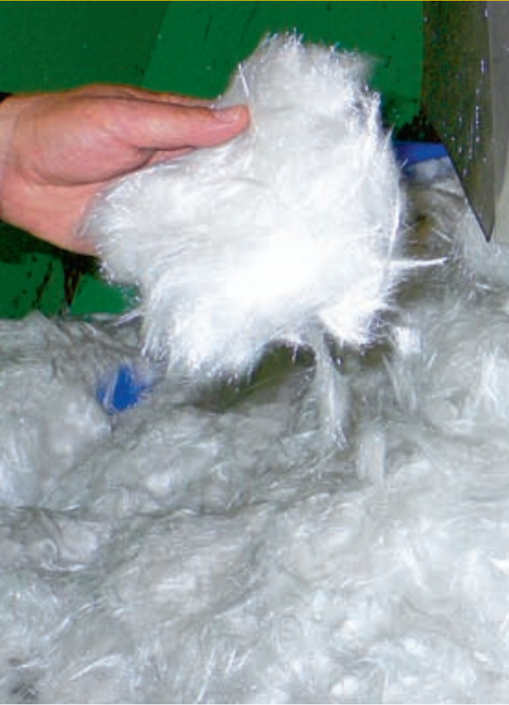
The fiberglass pictured is used in manufacturing the hulls of these boats.
