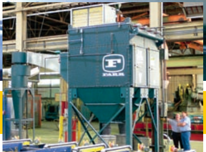
GS16 on zinc arc spray
