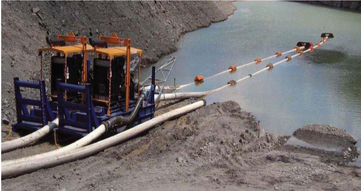
Figure 2-3 Example of Shore Based Pumping System with Floating Intake (Cornell Pump Company)
