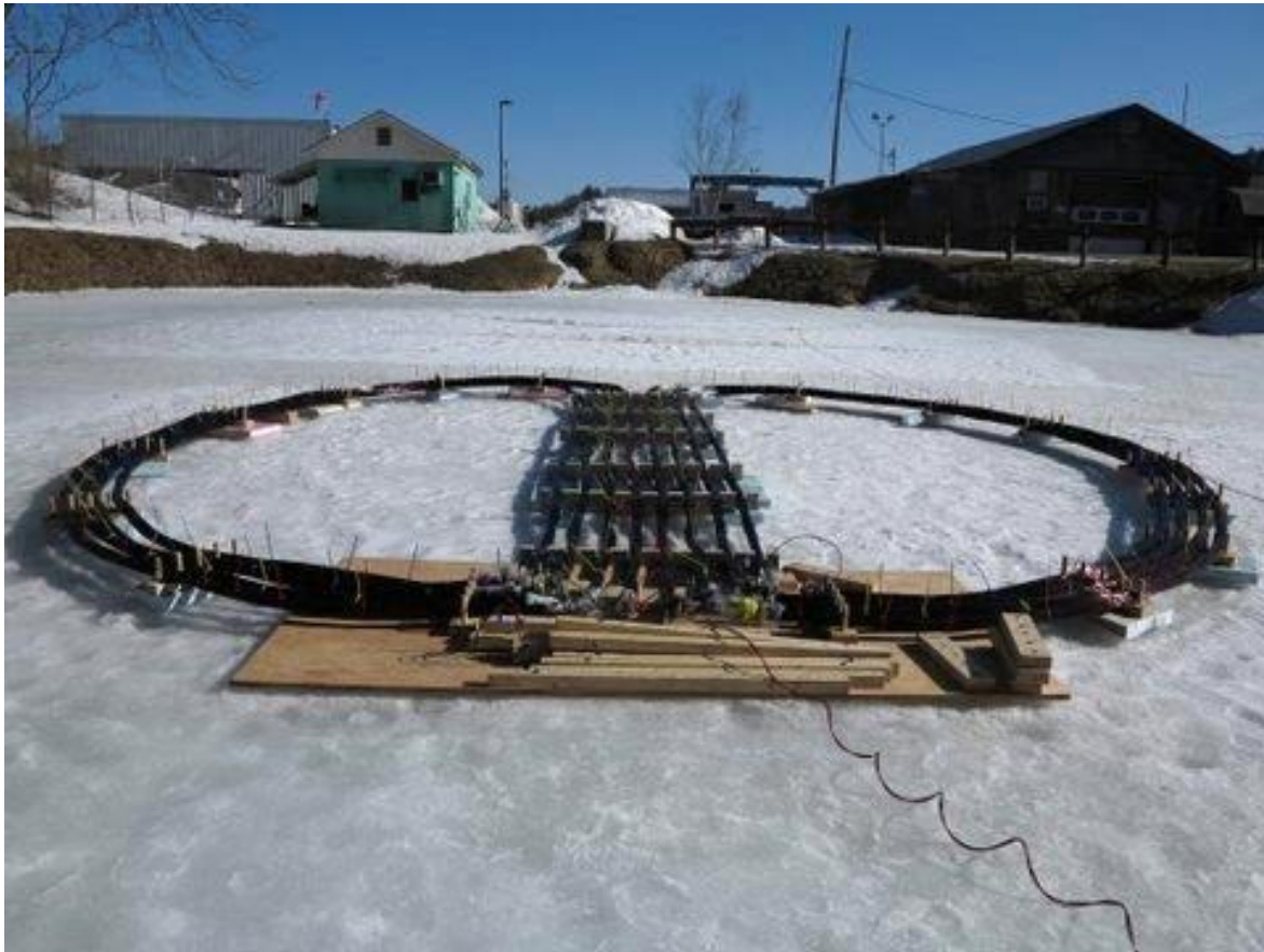
Photo 8 Experimental Prototype EFNMR Coil
