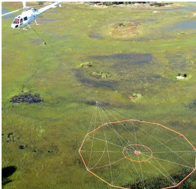
Photo 10 Example of a Helicopter Deployed Geophysical Sensor
