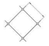
3.71.2 mesh length whole mesh distance between the centre of two opposing knots/joins in the same mesh when the mesh is fully stretched [NS-EN ISO 1107]
