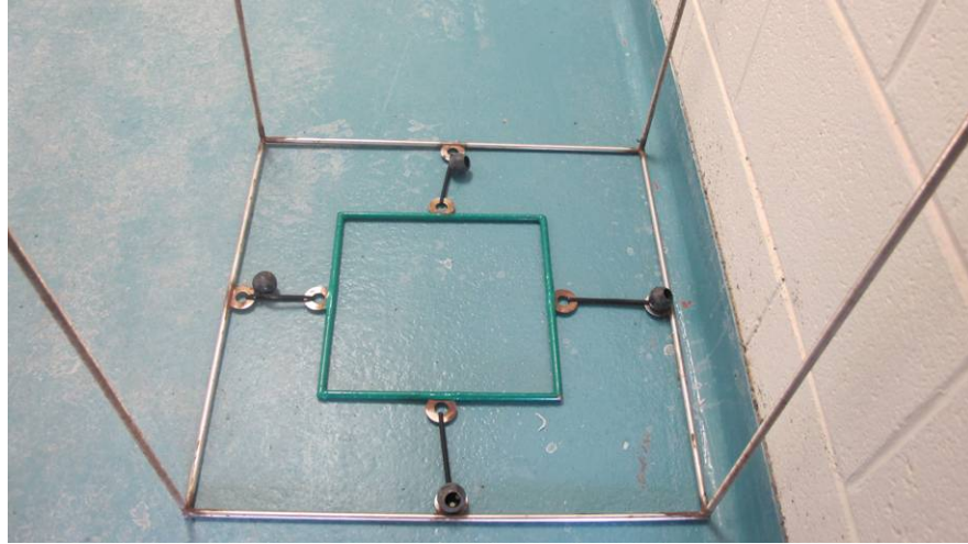
Figure 4: Bottom portion of the cage frame containing the 25x25cm green grid
