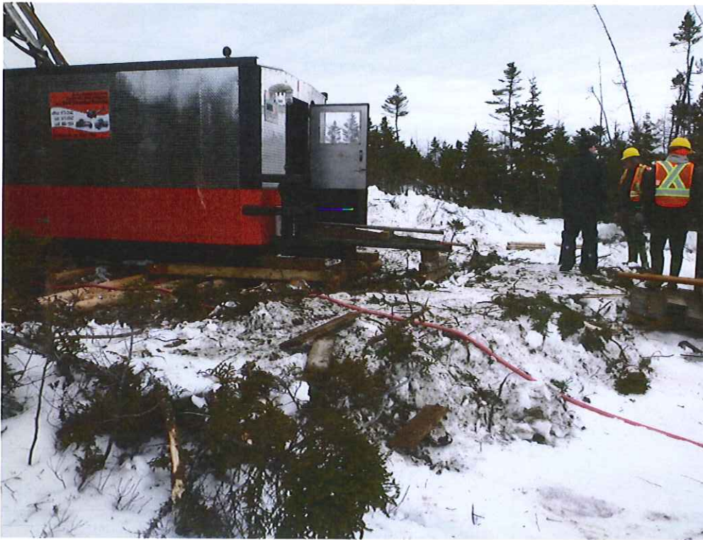
Figure 4. Active drill site prepared as described under point 1. Note the berm (foreground) consisting of mixed earth and organic cover, including slash. Frozen pond located out of picture to right.
