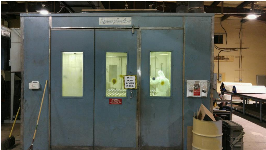
Spraybake Paint Booth, 14'2" x 24'2" x 10', Model No. SB10DDSMG, 220 Line V, 110 Control V, 3 phase, 60 Hz, 15 HP, max rating 650000 BTUH
