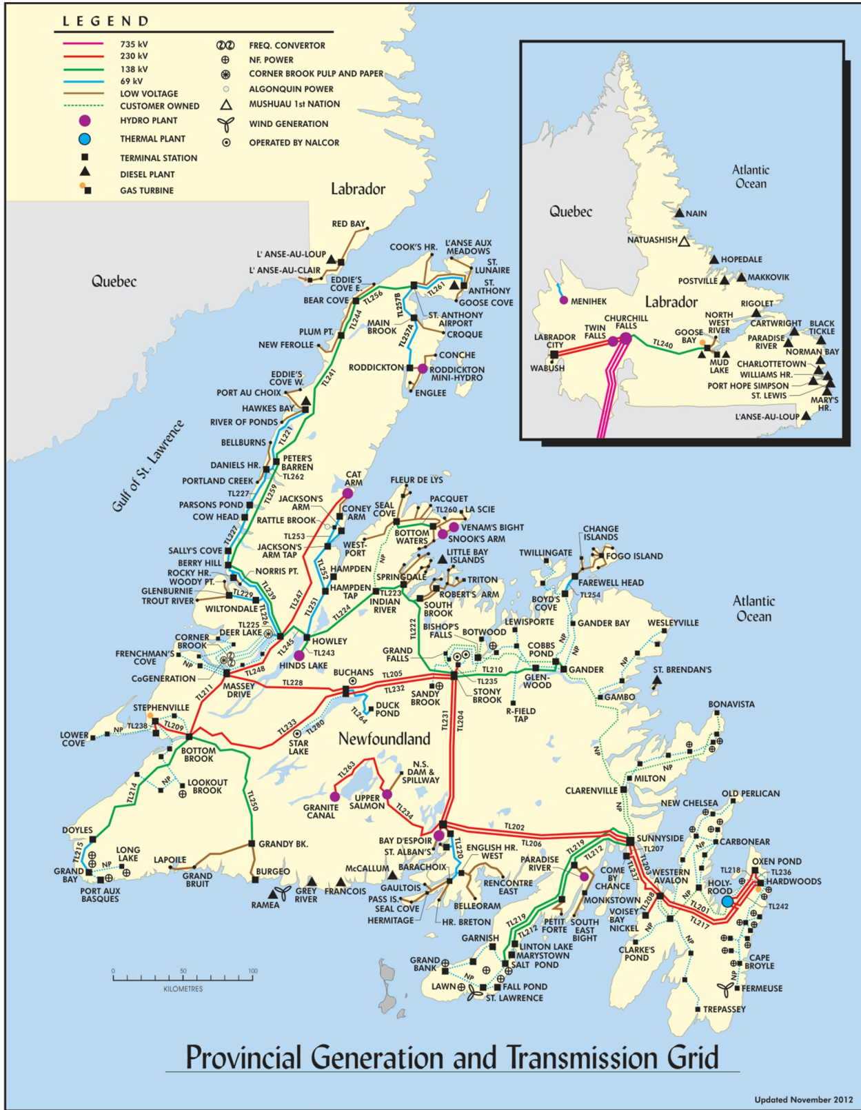
Figure 1.4 Existing Newfoundland and Labrador Generation and Transmission System
