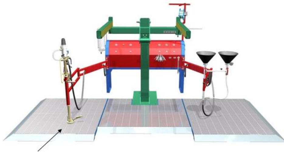
1. Impermeable Floor Any wasted fluid is Contained
