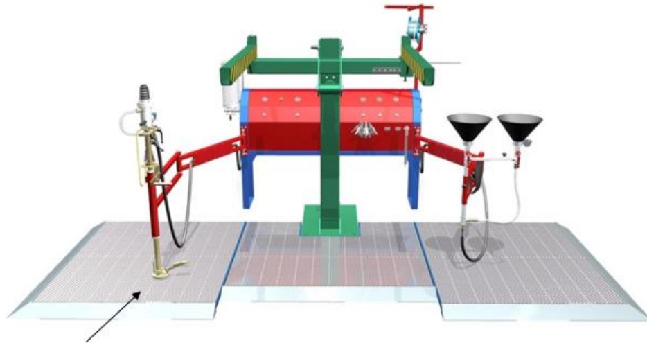
1. Impermeable Floor Any wasted fluid is Contained
