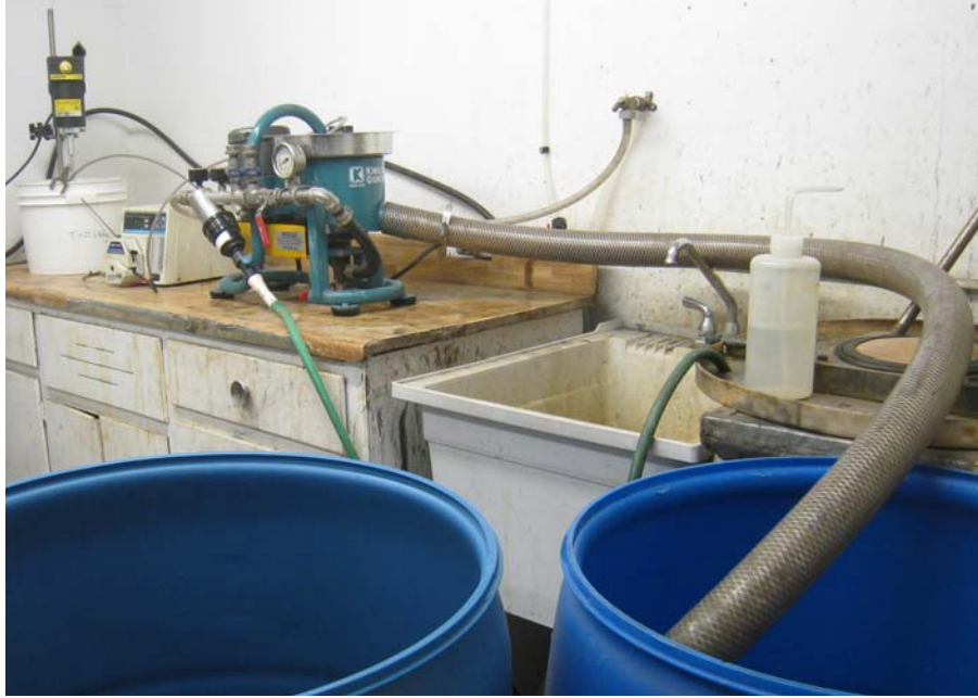
Figure 4: Bench Scale Knelson Concentrator.
