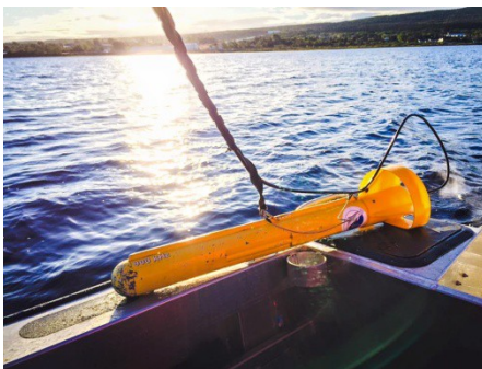
Figure 6: This "towfish" is pulled behind the boat.
