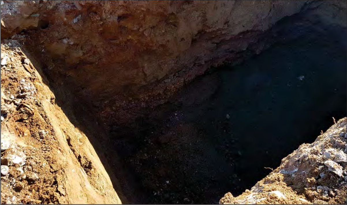
Figure A5 Test pit P2-3 soil layers and exposed pit bottom.
