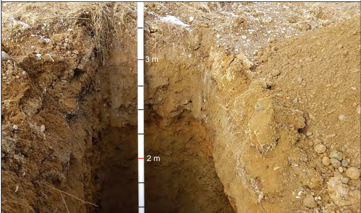
Figure A8 Test pit P3-1 scale, depth and sides of test pit. Note the vertical nature of the pit walls.
