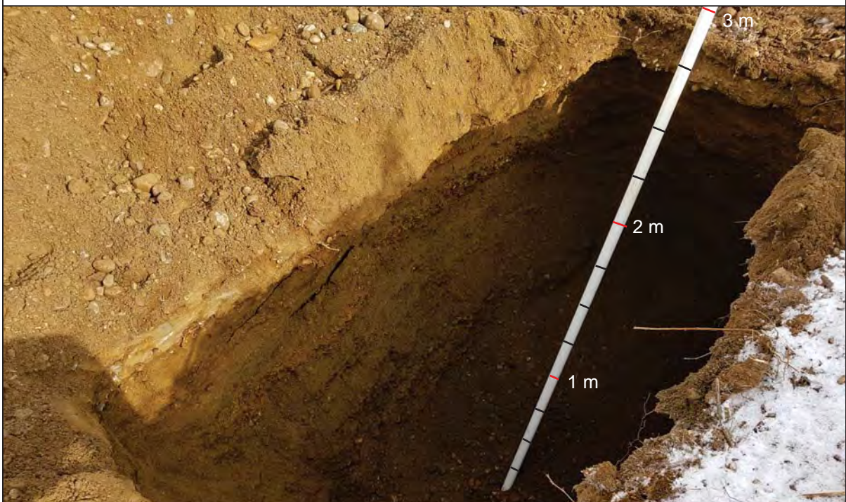
Figure A10 Test pit P3-3 scale, depth and sides of test pit. Note the coarse gravel layer near the bottom of the pit.
