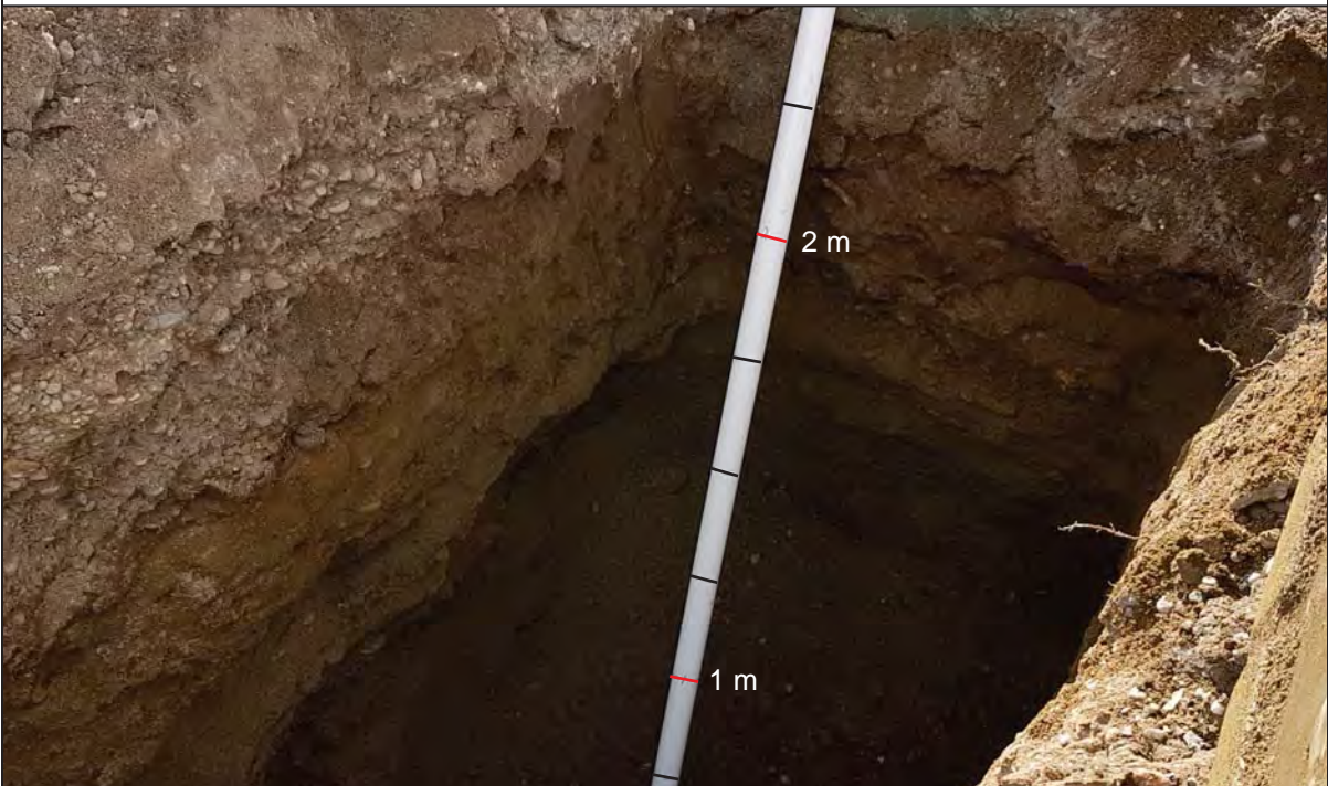
Figure A6 Test pit P2-4 Scale and sides of test pit. Note the coarse pebble to gravel layer near the surface.
