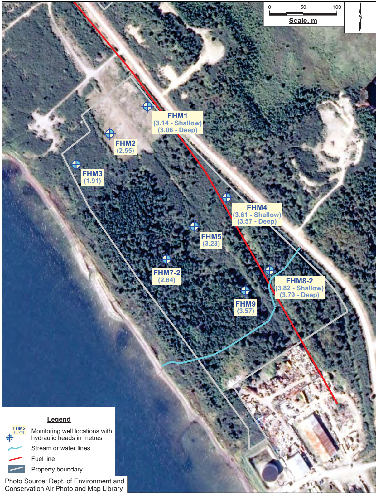
Figure 6 Measured hydraulic heads from the eight monitoring wells at the MHAC site.
