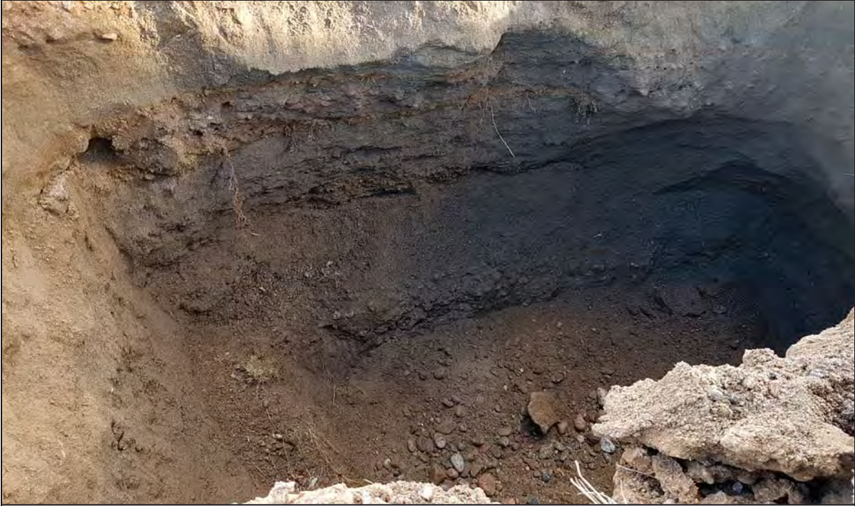
Figure A3 Test pit P2-2 soil layers in the pit wall and exposed pit bottom.
