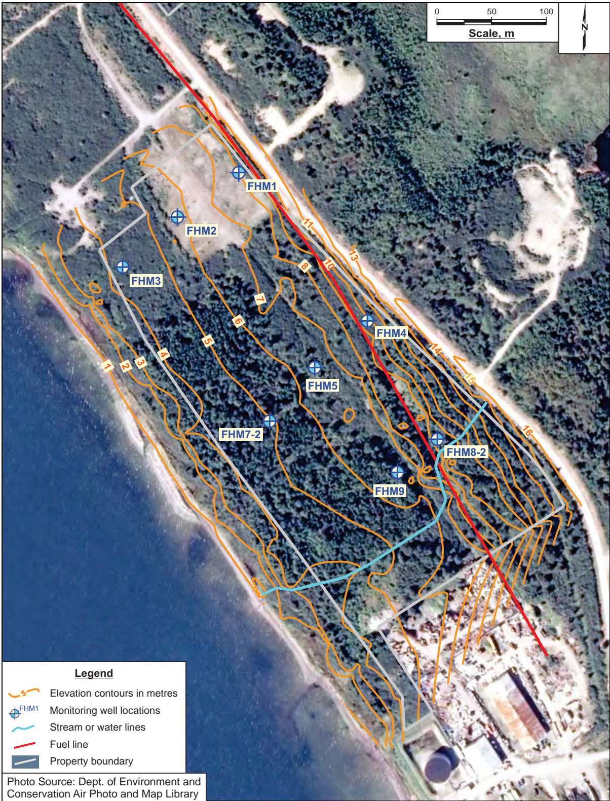
Figure 5 Elevation contour map of MHAC site based on topographic survey by Enos Fudge Surveys.
