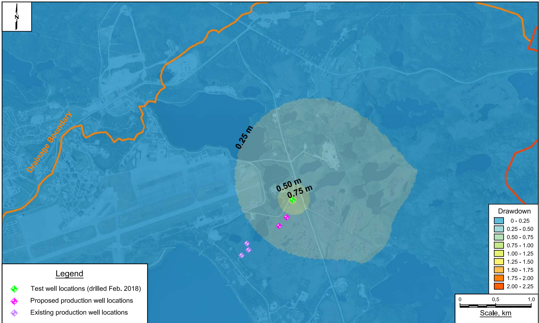
Figure 15 Capture area predicted by the model for a scenario of pumping the Test Well, MHPW1, at 1,820 Lpm, steady-state.
