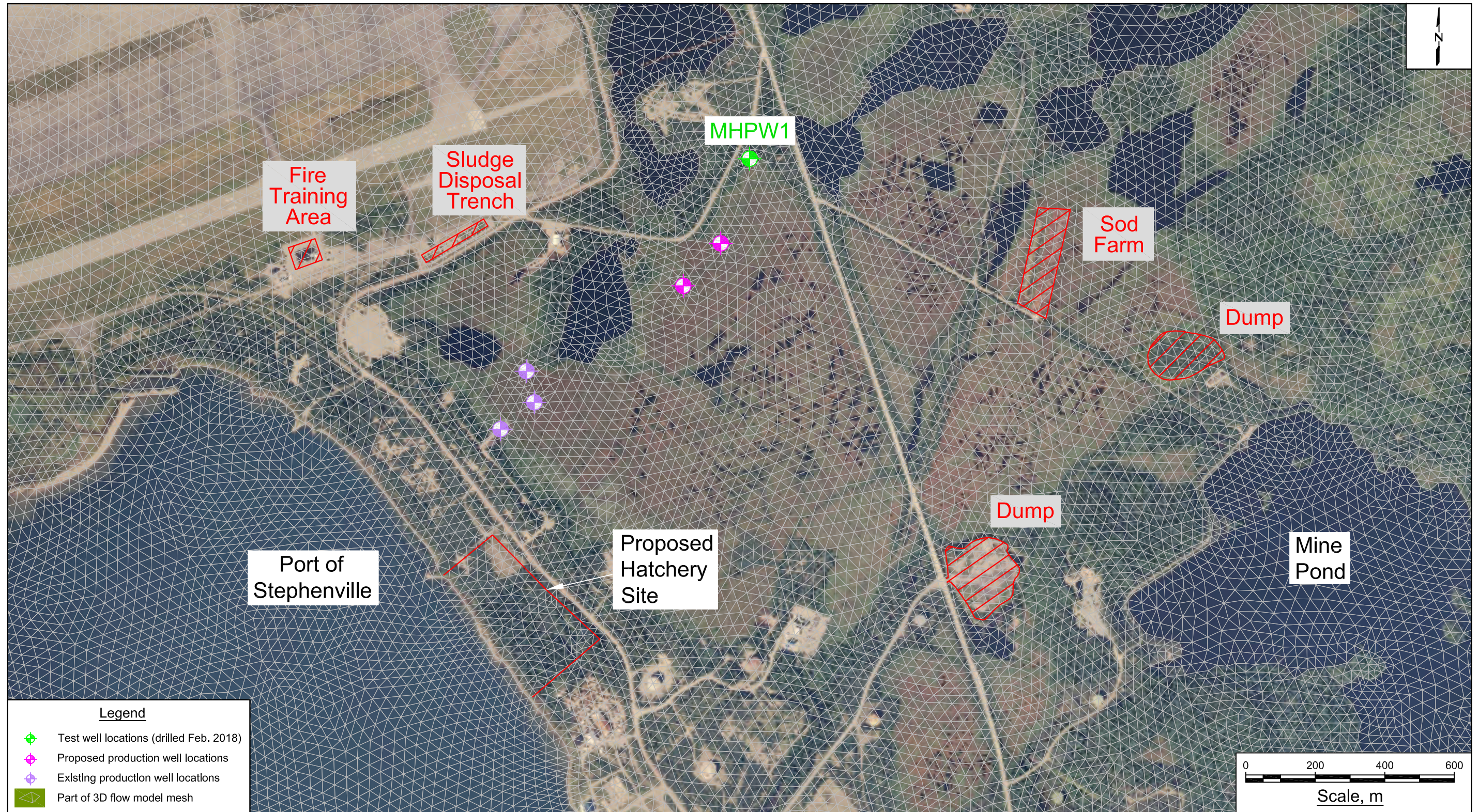
Figure 5 FEFLOW mesh (plan view) in the area of production wells (existing and proposed) with features incorporated in the 3D flow model.
