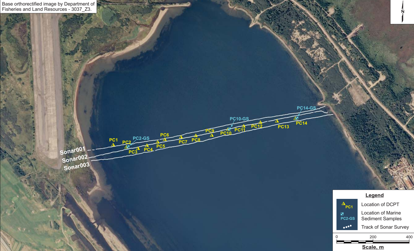
Figure 3 Track of the sonar survey along the proposed location of the pipe lines and location of dynamic cone penetration tests (DCPTs).
