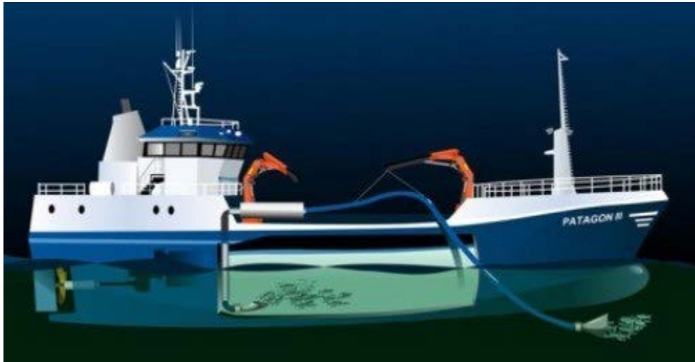
Figure 20: Typical Well-boat Configuration
