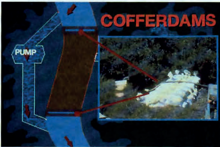
Figure 4.33 Cofferdams can be used in conjunction with temporary diversion channels to create a dry work area.
