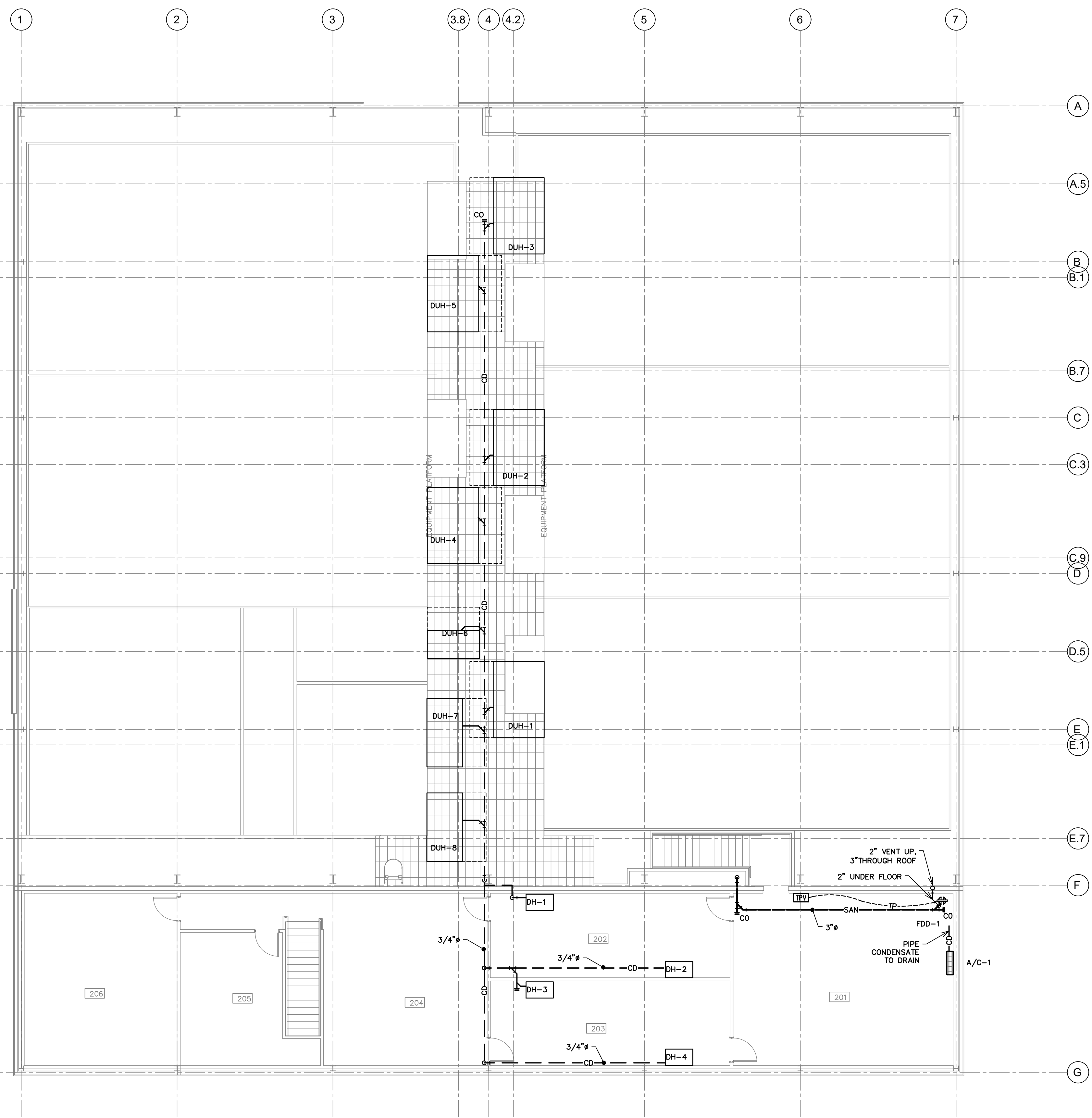
1 MEZZANINE FLOOR PLAN - SANITARY PLUMBING
