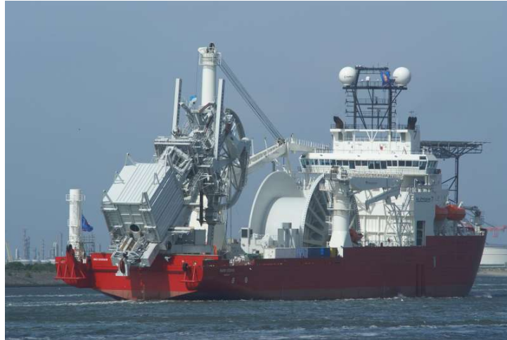
Figure 12: Seven Oceans Pipe-Laying Vessel ( http://www.shipspotting.com )
