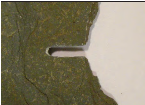
Closeup of saw mark on roof slate waste fragment.
