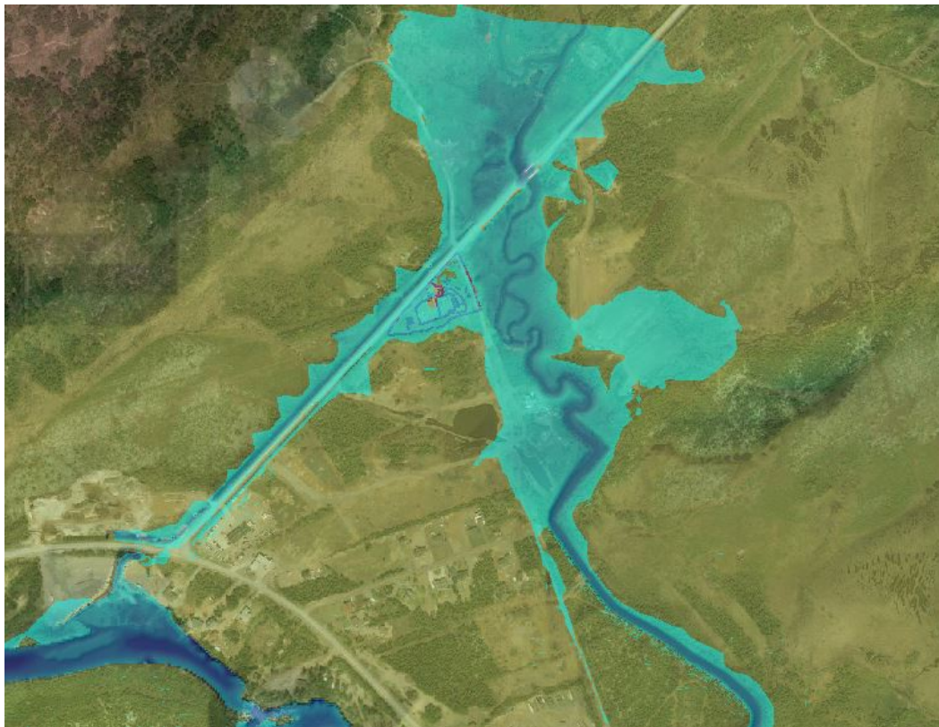
Figure 36: Option 2: 3.0m wide Ditch with 1200mm Culverts
