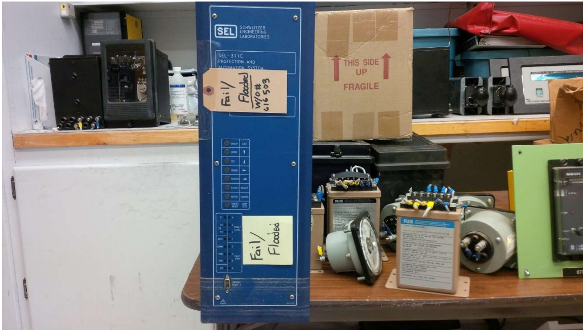
Figure 11 Relay Switch Removed after 2015 Flood
