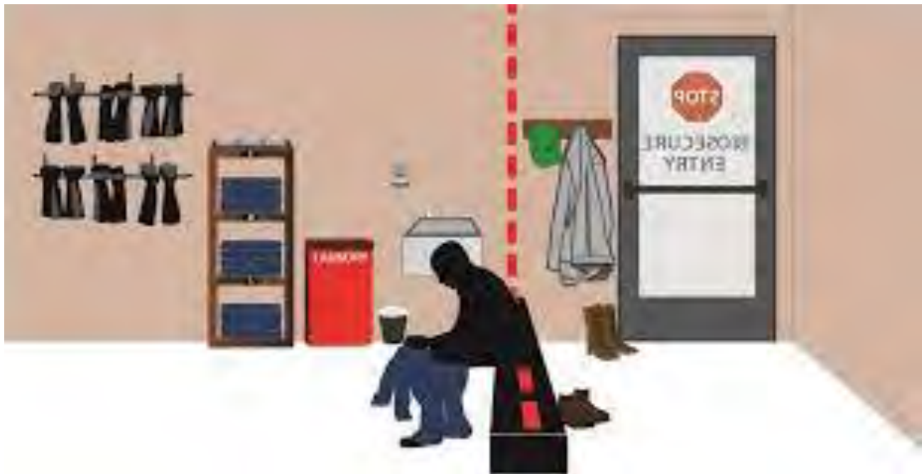
Figure 8: Primary Hygiene Room. Example of dirty and clean zone for Biosecurity. Dirty on the right and clean on the left.
