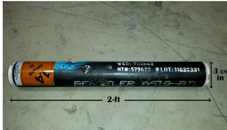
Figure 18. Jet perforating gun
