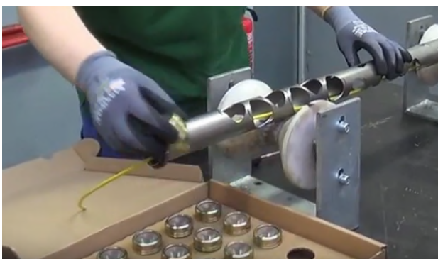
Figure 16. Installation of shaped charges
