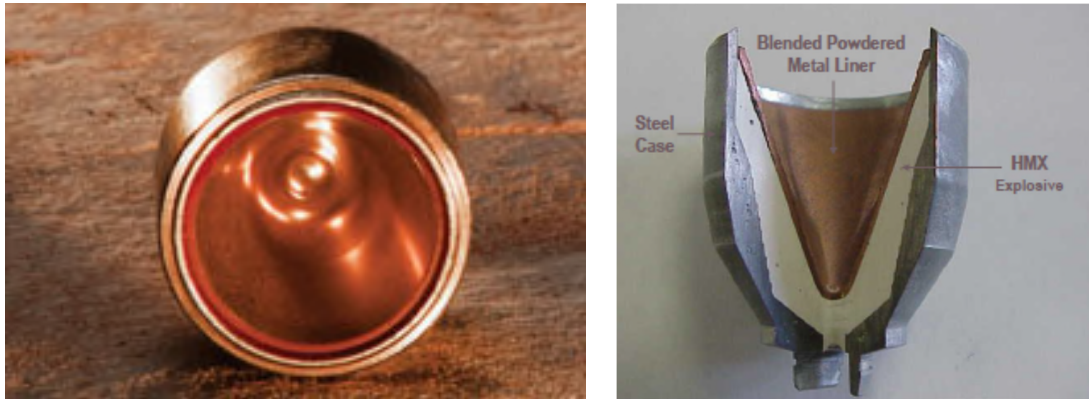
Figure 10. Shaped charge and cross-sectional
