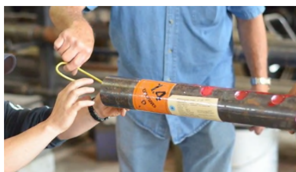
Figure 17. Installation inside hollow carrier
