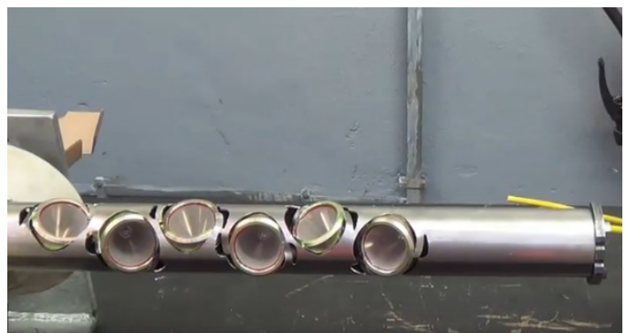
Figure 16. Installation of shaped charges
