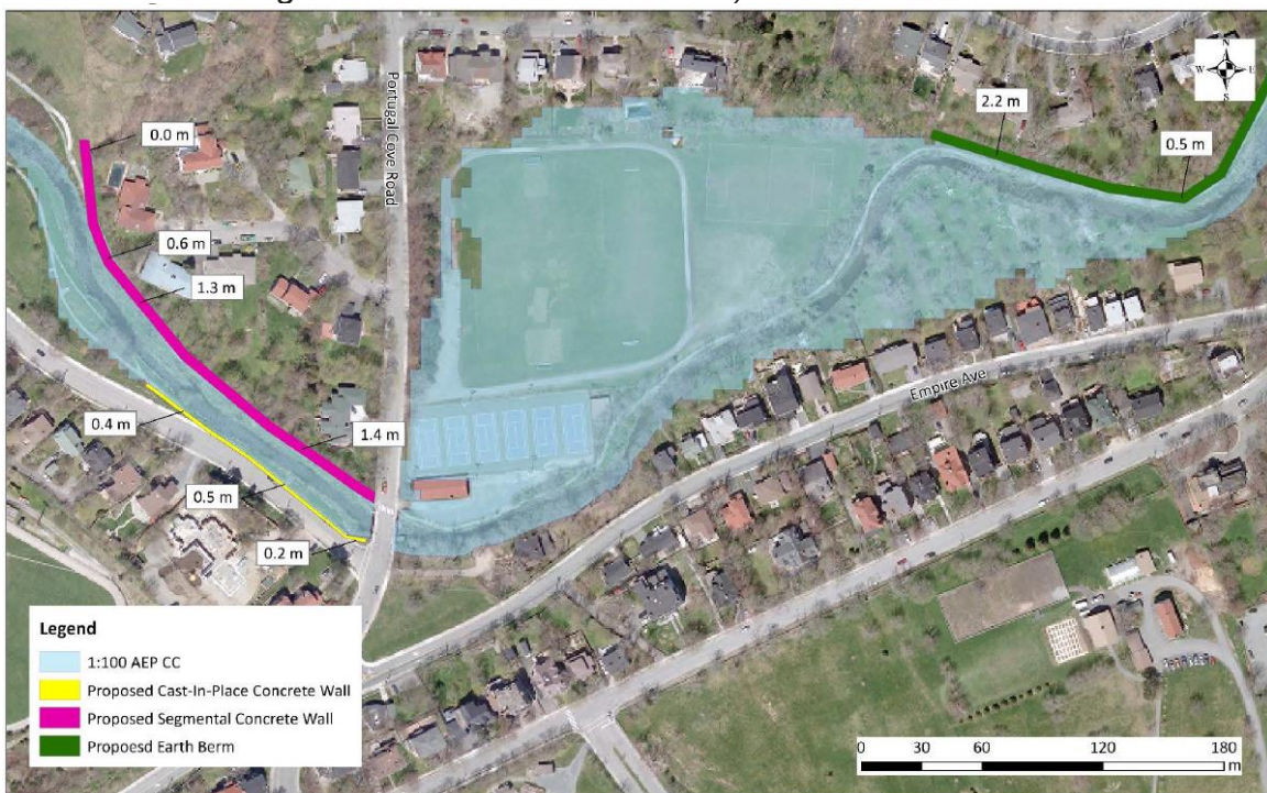
Figure 4: Wall / Berm Heights Per Alternate Project Phase Sequence (Maintain Status Quo – Long Pond Weir Not Constructed)
