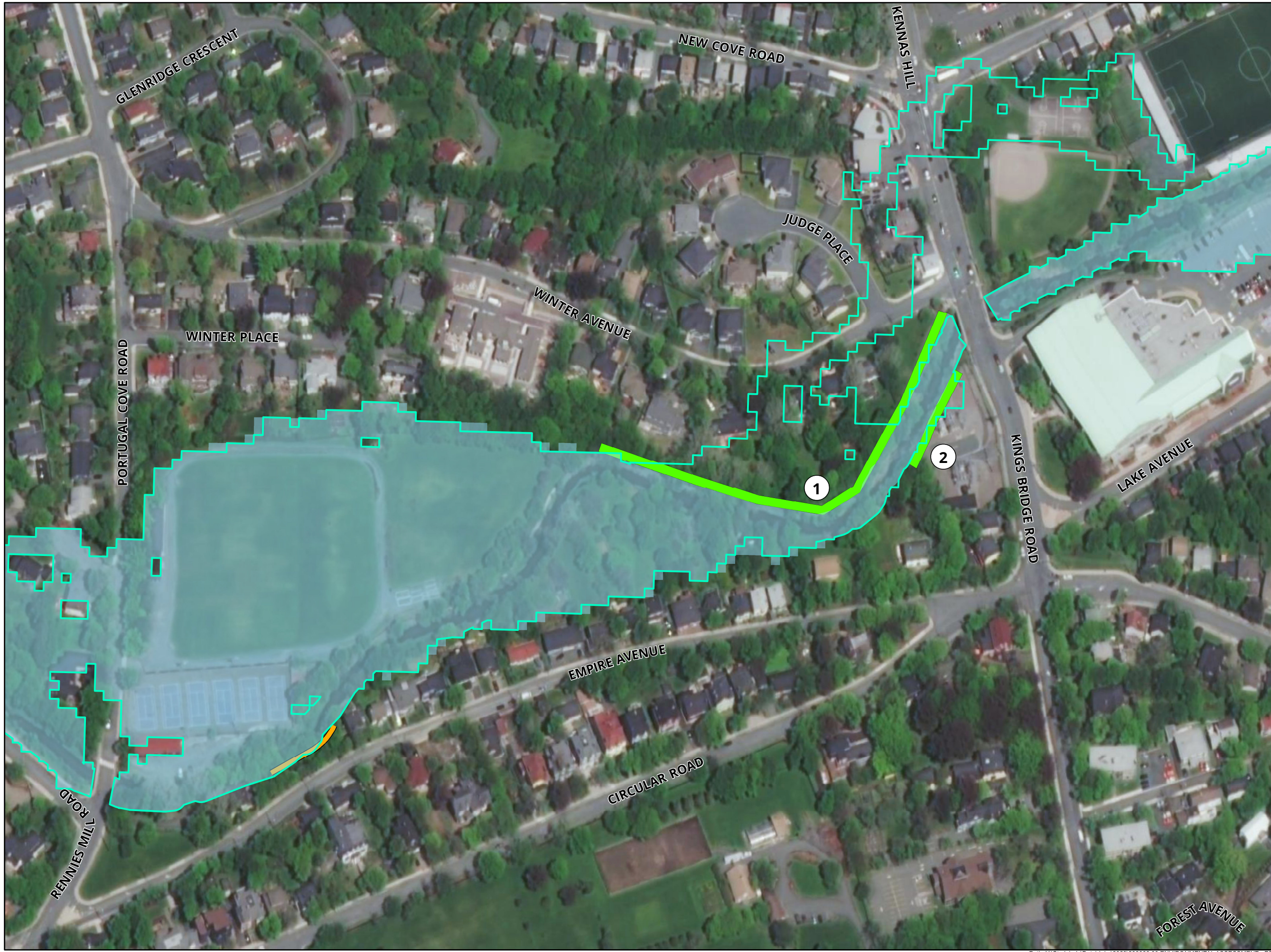
Figure 3.5: 1:100 AEP Climate Change Boundaries and Post Berm Construction
