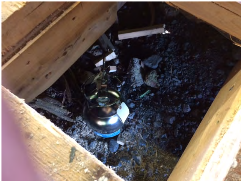
Photo 6 – View of the ambient air sample collection Suma canister in the access hatch of the Workshop during the September 2018 sampling event.
