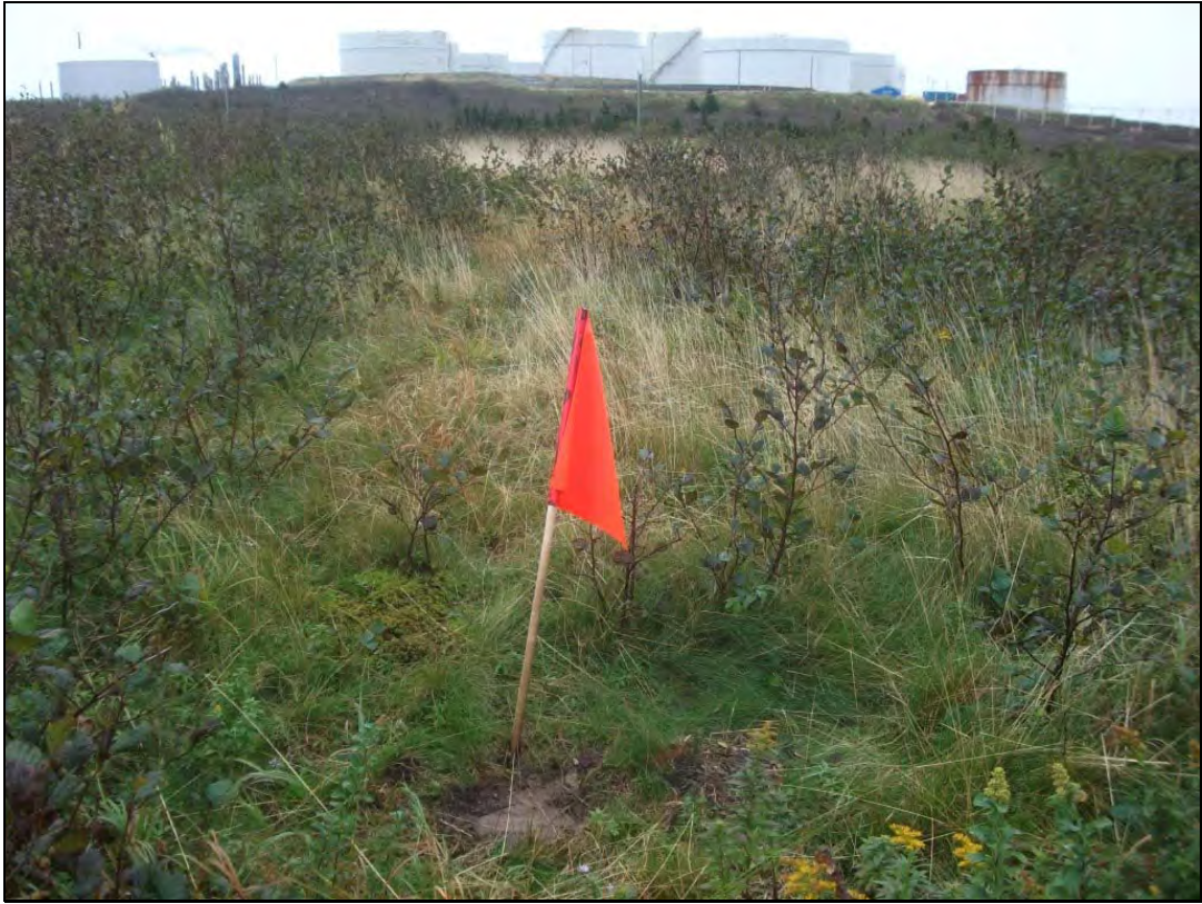
Photo 7: View, looking east, of a typical elevational survey control point installed on the landfill cover.
