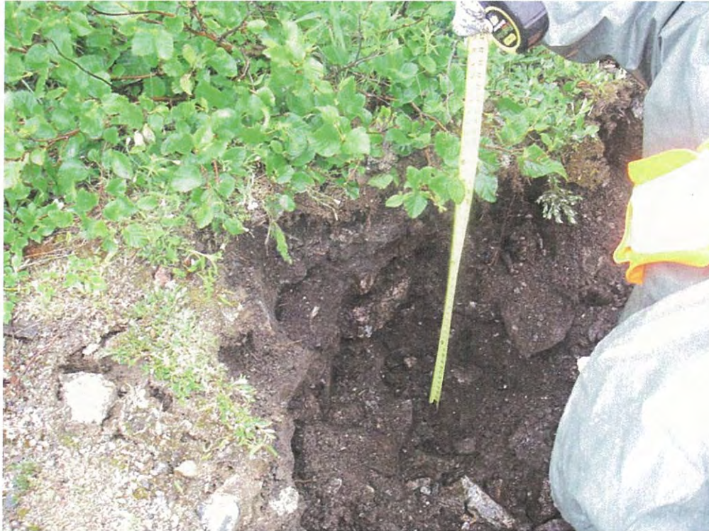
Photo 21 View of test pit depth measurement at the Main Base site
