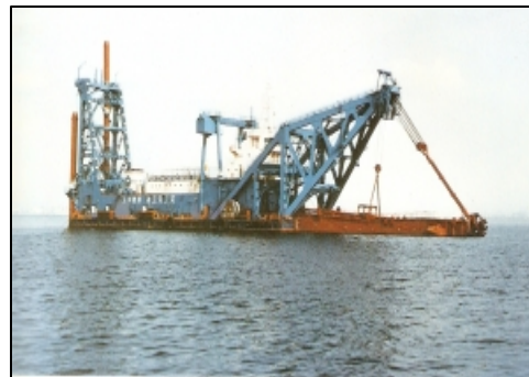
Photo 7 Cutter Section Dredge
