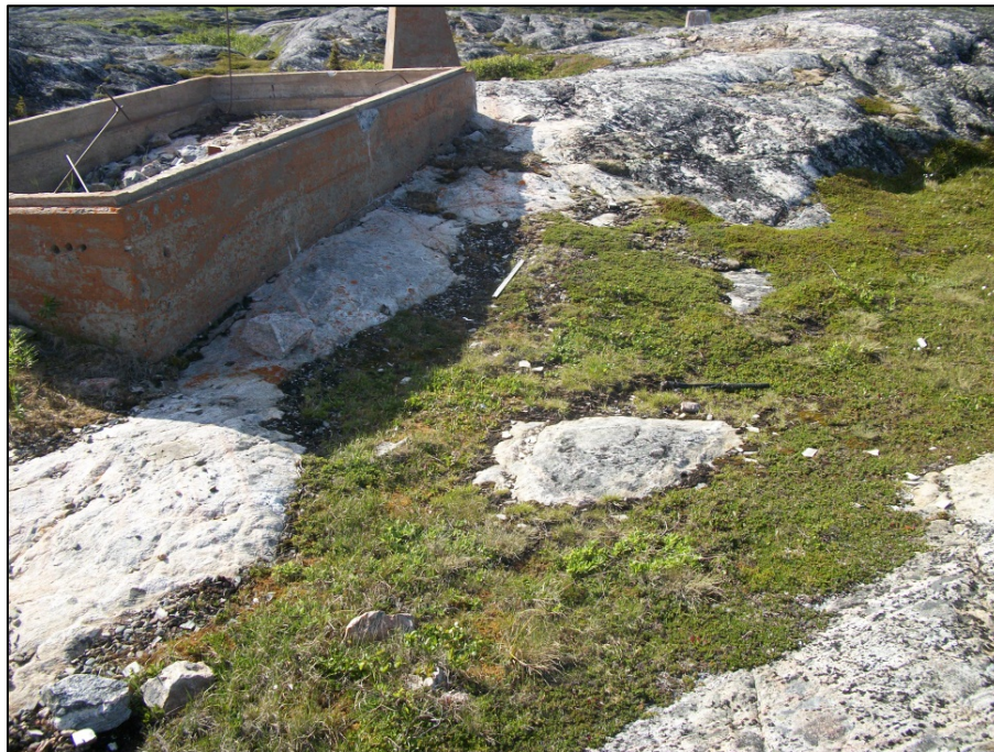
Photo 2. Area of cadmium, chromium and lead-impacted soil requiring remediation (MCL-BS10 and BS135), looking west.
