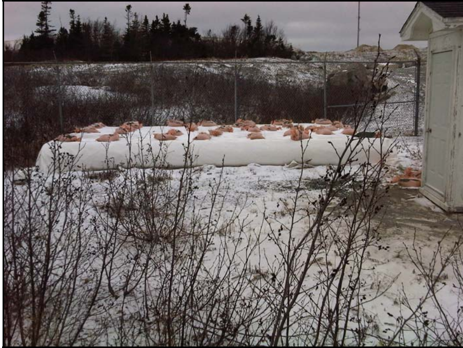
Photo 15: Stored LLDPE geomembrane: north side of secure enclosure.
