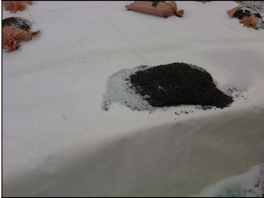
Photo 17: Destroyed sand bag.
