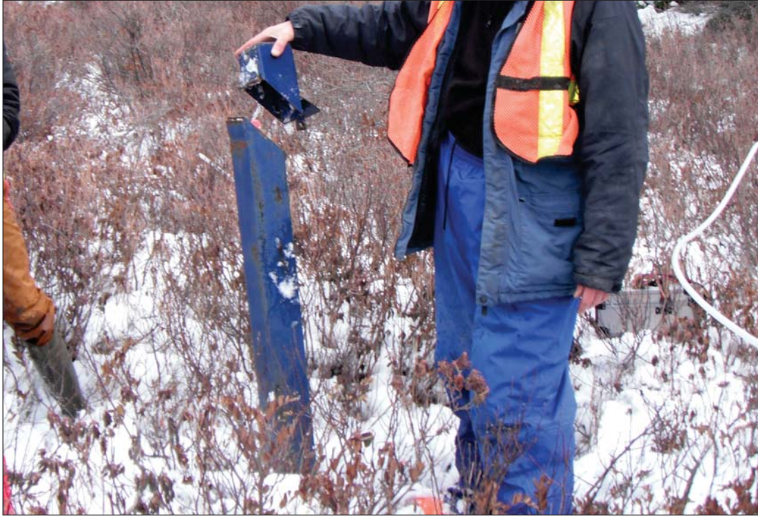
Photo 9 View of MW-07 during the December 2015 sampling event, showing the broken protective casing cover.
