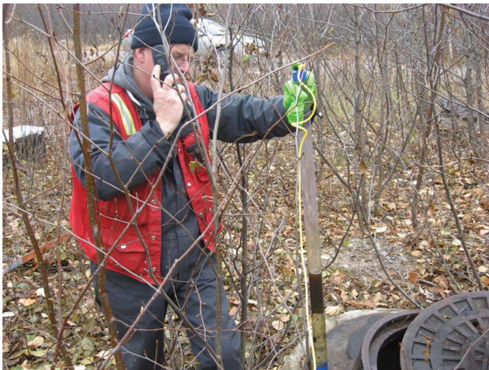
Photo 3 View of the second manhole being sampled. Note: 6 inches of product (09-Product1)
