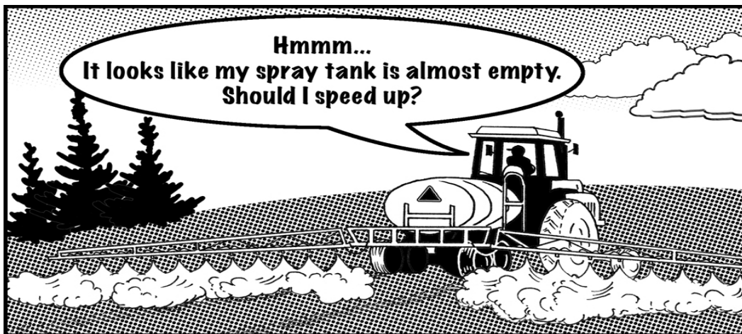
Figure 8-1: Always keep speed constant to ensure even distribution.
