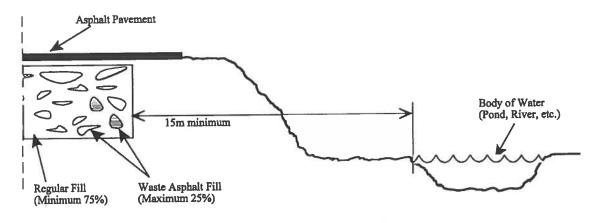
Figure 3: Permitted waste asphalt fill extent with respect to a body of water. Roadway perpendicular to water.
