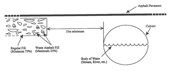
Figure 4: Permitted waste asphalt for road shoulder material extent with respect to a body of water. Roadway parallel to water.
