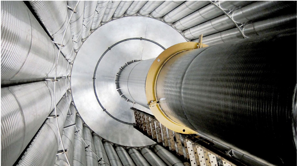
Figure 2.1 TOPSOE™ S-300 Ammonia Converter
