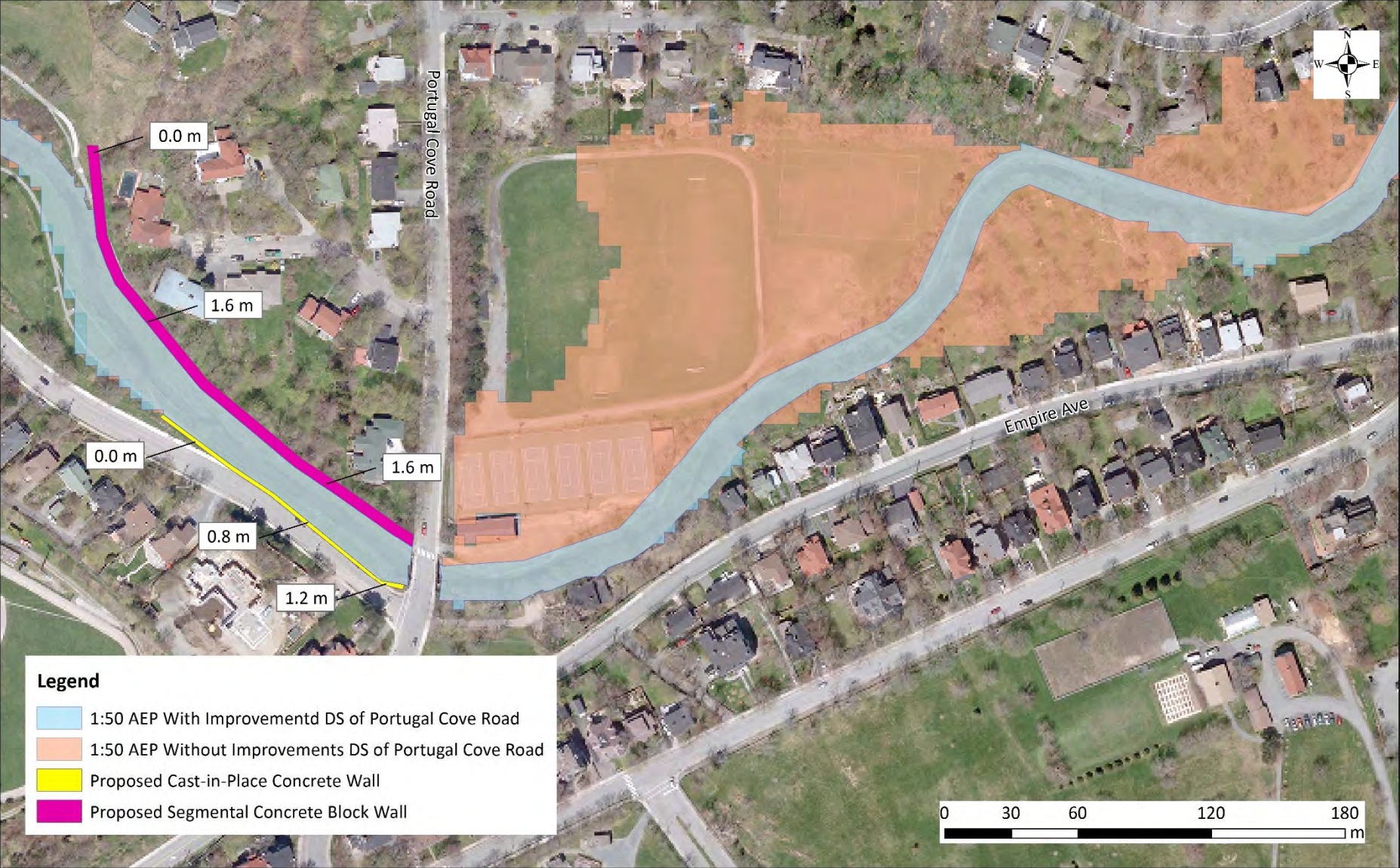
Figure 1: Comparison of 1:50 AEP Floodplains With and Without Improvements Downstream of Portugal Cove Road
