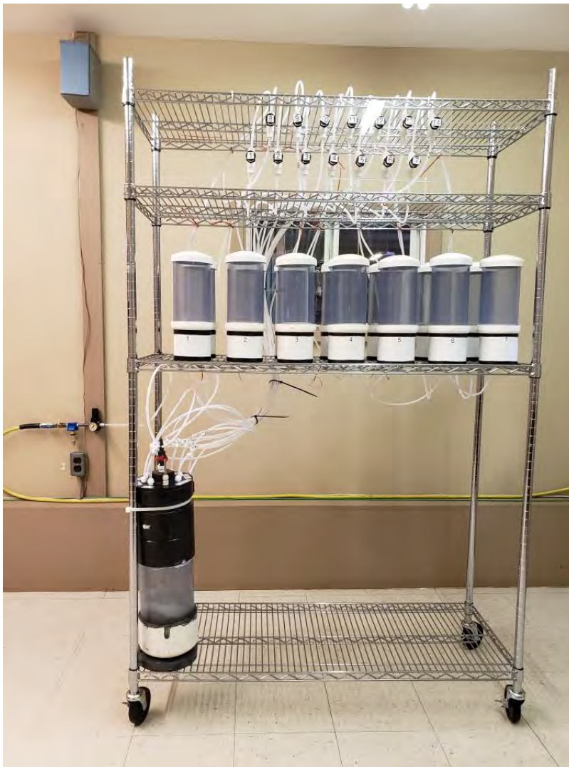
Figure 54: ARD – Humidity Cell at RPC Laboratory
