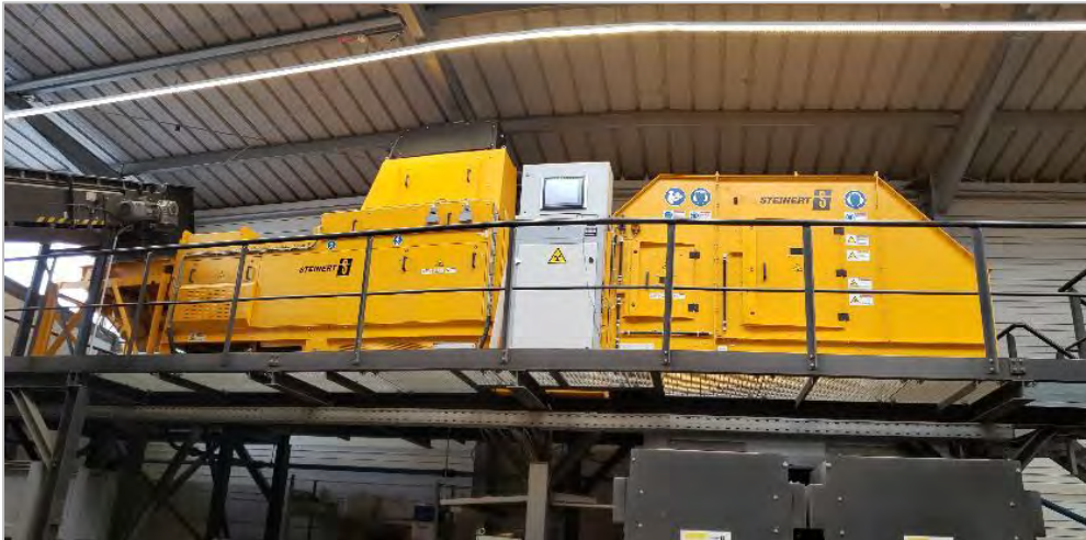
Figure 11: Pre-Concentration X-Ray and Laser Equipment
