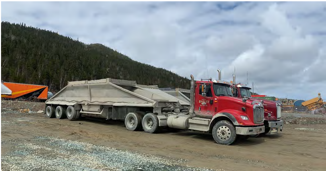
Figure 16: 30 Tonne Haul Truck for Ore Transport to Nugget Pond Mill
